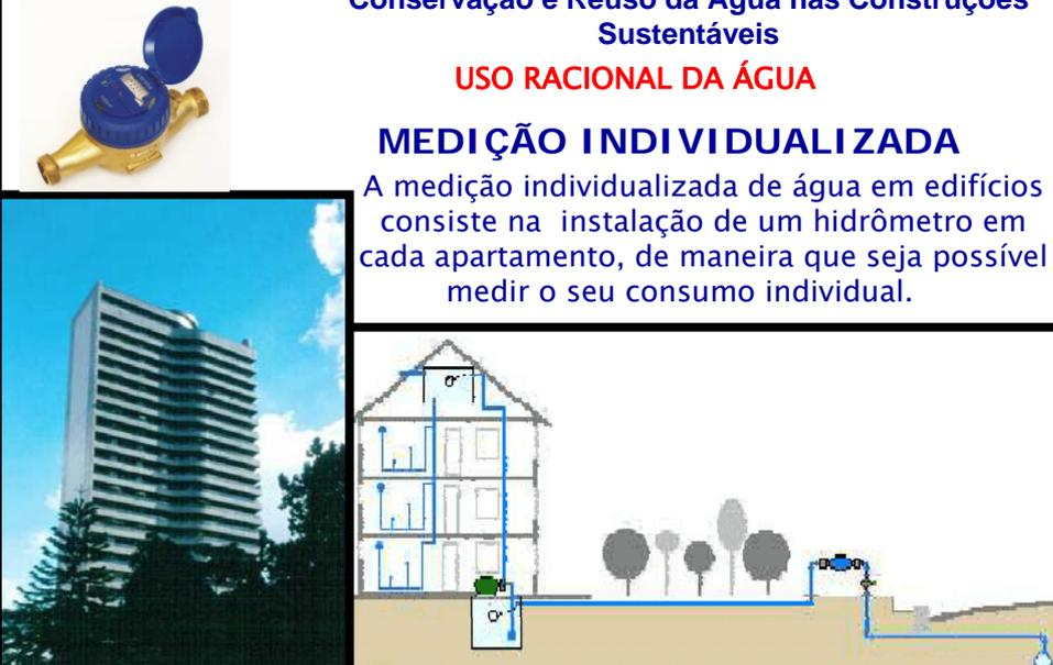
The image contains three main visual elements: a close-up of a blue and brass water meter; a photograph of a modern high-rise apartment building; and a cross-sectional diagram of a building showing individual water meters installed for each floor and unit, connected to a central water supply system.
