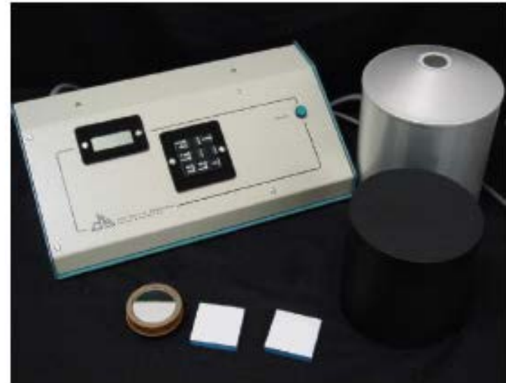
Solar Spectrum Reflectometer (ASTM C1549)
